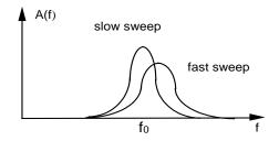
In a spectrum analyzer it is also possible to set the sweep time. If the scan is too fast, the output of the filter may not reach its maximum value causing distortion in the output signal. This behavior is shown in the figure for a sinusoid.
