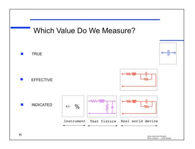
Before proceeding to practical measurements, we need to understand the concept of True, Effective and Indicated values. This is essential since we all tend to forget that the instrument does NOT necessarily measure what we want to measure. By the way, which value do instruments measure?
