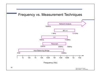
This chart will help you visualize the frequency range for 5 measurement techniques. The frequency range numbers are a mix of practical and theoretical limits and should be used as a reference only. The autobalancing bridge basic accuracy is 0.05% while the network analysis one is 1.5%. This already uncovers possible trade-offs.
