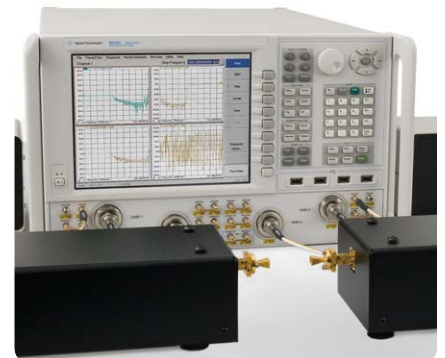
Direct connection of VDI modules to a 50 GHz PNA-X enables S-parameter measurements to 1.05 THz.
