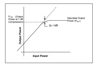
NOTE: Most amplifiers start to compress approximately 5 to 10 dB below  $P_{1dB}$ . Applying signal power levels above this point results in a decrease in Gain – therefore, the change in output power will not be linear with respect to a corresponding change in input power to the point where the amplifier is at saturation ( $P_{SAT}$ ) and the gain equals zero.
