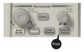
The oscilloscope is now set in the default configuration. Because the oscilloscope may have been used in a variety of applications by a variety of people, it is a good measurement procedure to put the oscilloscope in a known starting mode (Default Setup). This will make it easy to duplicate measurements as no special conditions will be set.
