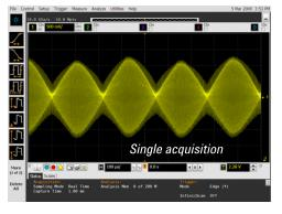
Adjust trigger level to approximately 3 volts, which is down approximately 1/3 below the highest peak. Using this level will provide potential re-arm times during the valleys of the envelope.
