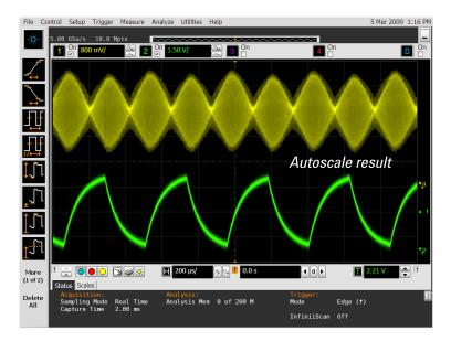
In this lab, a stable trigger is accomplished by triggering on the synchronization signal on channel 2. In the absence of a synchronization signal, trigger holdoff can be used to achieve a stable trigger (see Appendix A).
