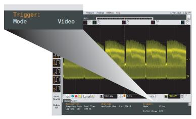
The trigger conditions are in the lower right corner of the display.
