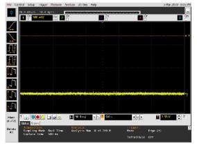
Auto mode forces triggers if the trigger conditions are not met and shows untriggered waveform activity.
