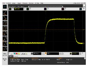
Trig'd mode waits for a waveform that meets the trigger conditions before displaying any activity.
