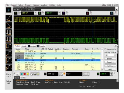
20 Click on either a Data 1 or a Data 0 packet row; then, select the Payload tab to see the packet contents.
