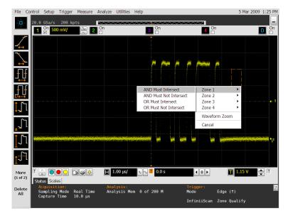
The oscilloscope now triggers and captures only waveforms where the glitch occurs.
