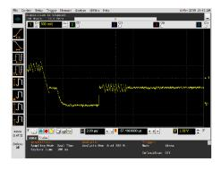
With deep memory, we are able to zoom in by a factor of 5.000 from the original waveform to analyze details of the color burst of this video signal.
