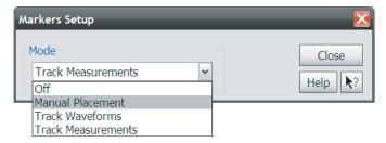
2 For example, in the Markers Setup dialog, select Manual Placement from the drop-down, and click **Close** (or press [Markers] again).
