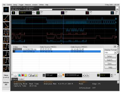
As you move the blue vertical marker in the waveform display, it tracks in the protocol viewer window.
