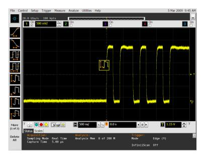
After dropping the measurement icon on a waveform, markers for the measurement appear on screen, and the measurement data appears in the bottom portion of the screen.
