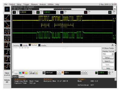
Move the mouse and see the X-Y coordinate information change in the Payload tab.
