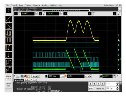
13 Use the forward, back, start, and end buttons to play through the acquired segments one by one.
