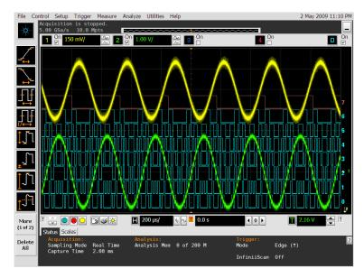
The channel 1 signal (yellow) is the filtered version of the output.
