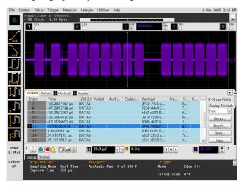
**32** Click on either a Data 1 or a Data 0 packet and click on the payload tab to see the contents.
