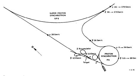
Fig. 1. Overall layout of the pp project.
