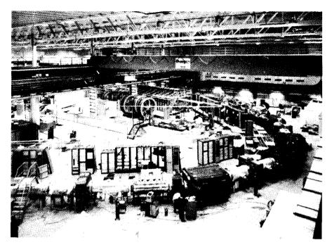
Fig. 15. View of the Antiproton Accumulator before it was covered by concrete slabs. The silvered material around the vacuum tanks is insulation, needed because everything may be heated to 300" to obtain ultra-high vacuum. The transmission lines crossing the ring and carrying the cooling signals may be seen.
