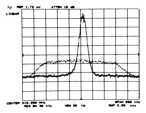
Fig. 13. Precooling 6 x 10° p̄'s in 2 seconds. Longitudinal Schottky band at the 170th harmonic (314 MHz) before and after cooling.
