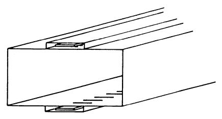
Fig. IO. Slot-type pick-up or kicker. One end of the transmission line is terminated with its own characteristic impedance.
