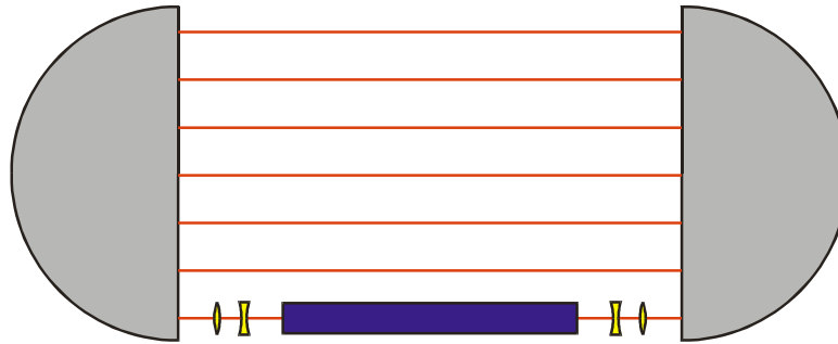
Fig. 11: Second focusing scheme in a racetrack microtron
