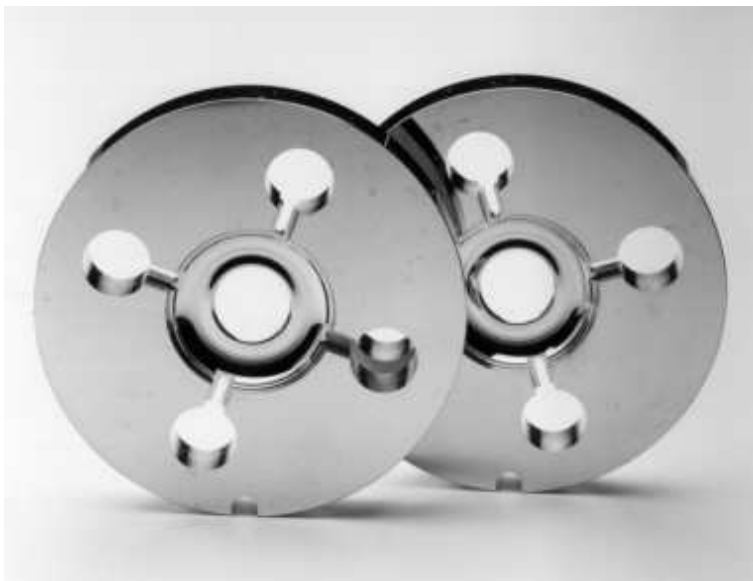
Fig. 2: Prototype diamond-turned disk of an NLC X-band accelerating structure. The four holes coupled to the accelerating cells are used for transverse wakefield suppression.
