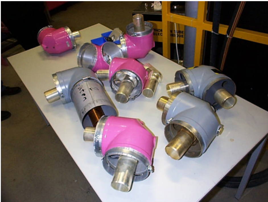
Fig. 2: Typical high-power coaxial components
