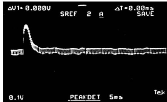
Fig. 8(b): Same as Fig. 8(a) but with the phase loop active. The synchrotron oscillation is completely damped within half a synchrotron period of 5 ms.
