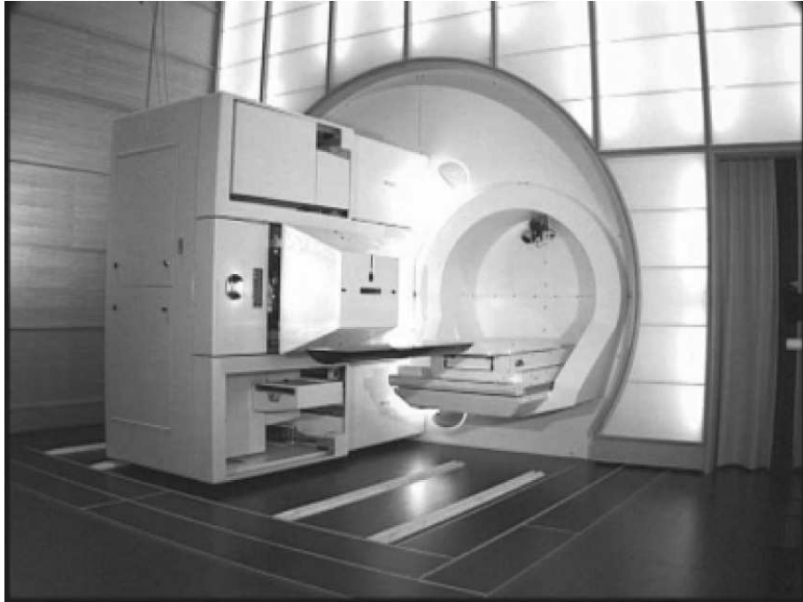
Fig. 7: Photograph of the PSI proton treatment room with the head of the compact gantry dedicated to proton beam scanning
