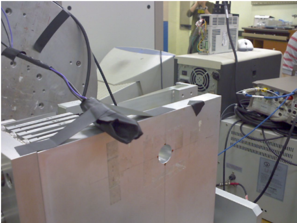
Fig. 1. The LYSO crystal detector system on the beam line.
